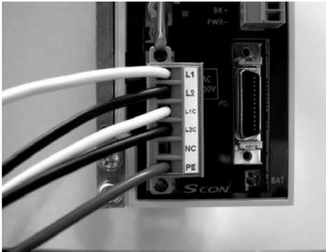
As shown to the left, tighten the screws to secure the connector.
