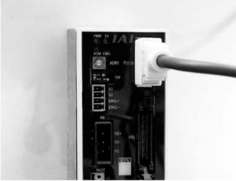
Use the pulse-train control cable when the controller is operated in the pulse-train input mode. It should not be connected when the controller is operated in the positioner mode.
