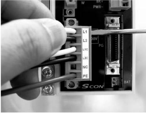
As shown to the left, insert the stripped end of the cable into the connector and screw in the cable using a screwdriver.
