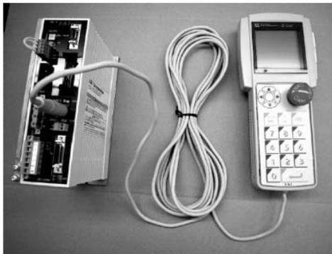
If the teaching pendant/PC software cable is used, connect it to the teaching connector on the controller.
