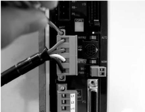
Use a screwdriver to tighten the screws at the top and bottom of the connector to secure the connector.
