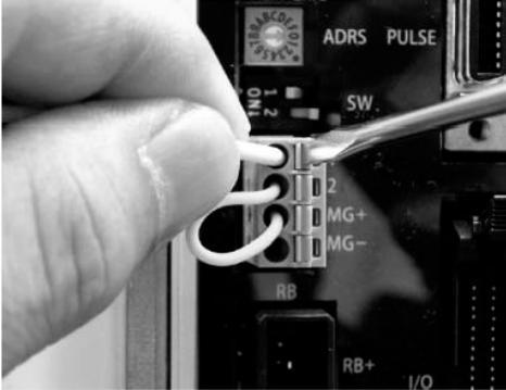
As shown to the left, insert the stripped end of the cable while pressing down the spring using a screwdriver.
