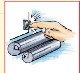
Shaft only turns a small amount each time the PB is pressed.
