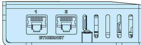
Figure 5-13 EtherNet/IP Connection for ACS Drive Programmability
