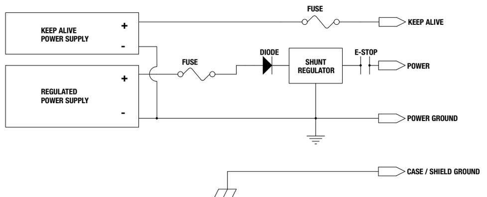
**Figure 6-17: Regulated Power Supply with Blocking Diode and Shunt Regulator**
