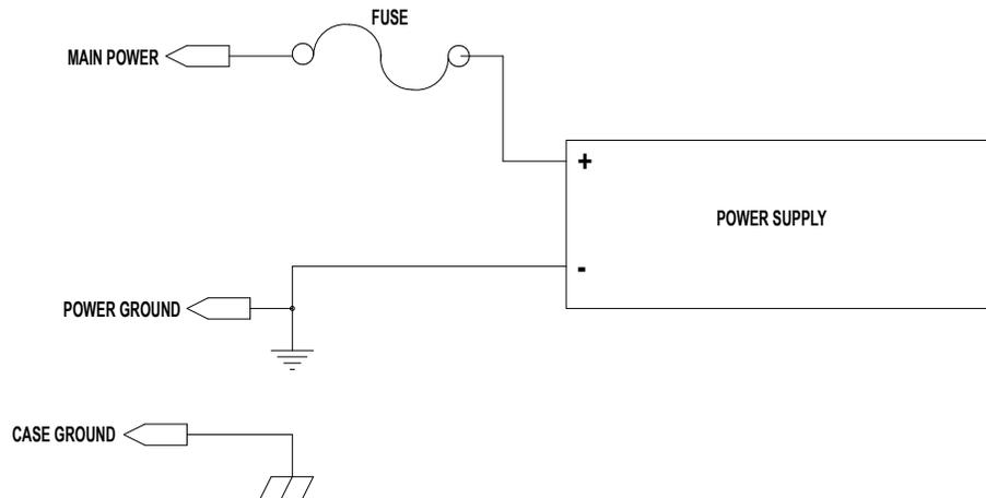
Figure 6-13: ACS Drive Single Supply – Main Power
