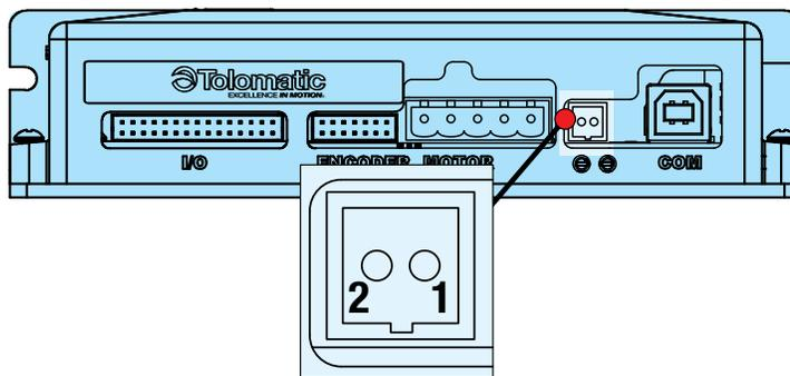
Figure 5-8: Brake Connection
