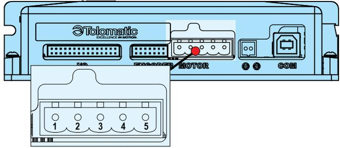
Figure 5-1: Motor Power Connection on ACS Drive
