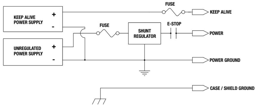
**Figure 6-15: Unregulated Power Supply Configuration with Shunt Regulator**
