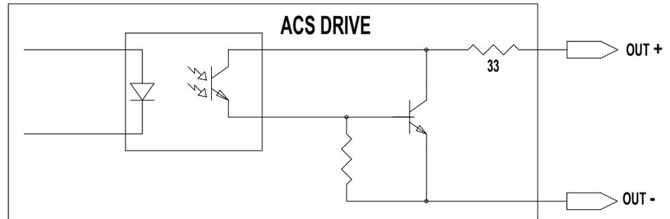
**Figure 6-6: Output Circuit**
