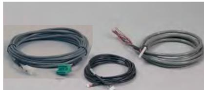
Tolomatic offers a motor power cable with drive and motor mating connectors, an encoder cable with drive and encoder connectors, and an I/O cable with drive mating connector to flying leads. Cables are available in 3, 5 or 10 meter lengths.
