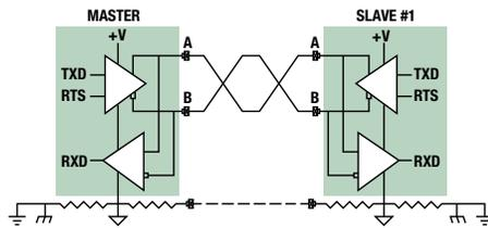
Figure 5-12: Resistors in ground wire to limit current
