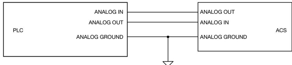
Figure 6-10: Analog Output Equivalent Circuit
