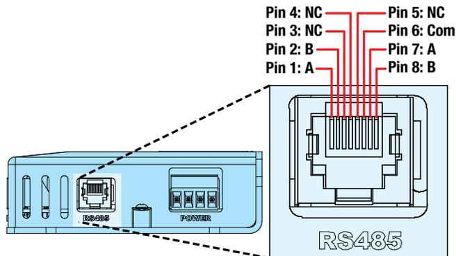
Figure 5-11: ACS 2-Wire RS485 with RJ45 Socket
