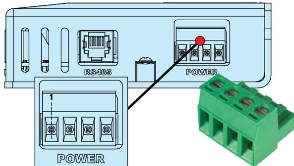
Figure 5-7: Input Power Connection
