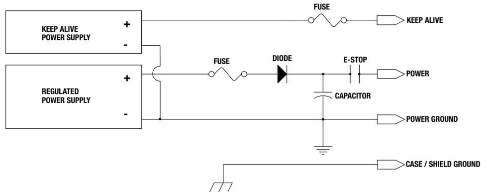
**Figure 6-16: Regulated Power Supply Configuration with Blocking Diode and Added Capacitance**
