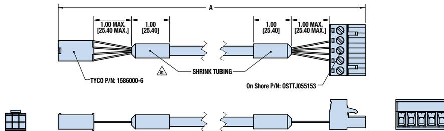
**Figure 5-2: Motor Power Cable 3604-1708/1709/1710**
