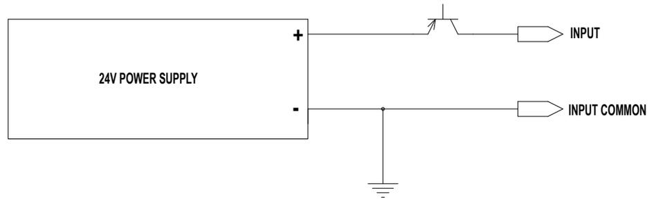
**Figure 6-3: Input Source (PNP) Connection**
