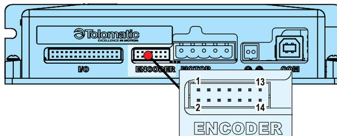
**Figure 5-3: Encoder Connection on ACS Drive**
