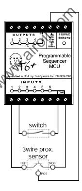
Electromechanical devices such as magnetic reed switches, limit switches, push button switches and pressure switches are wired with no regard to polarity (positive/negative).
