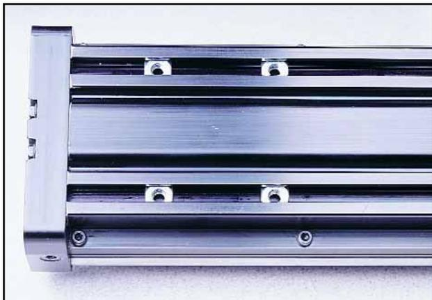
Base mounting linear slides may be accomplished by fastening directly to "T" slot nuts provided in the base of the slide or by using the base mounting plates shown below. These plates are also used as a mounting surface when using tube supports (see chart at the bottom of this page).
