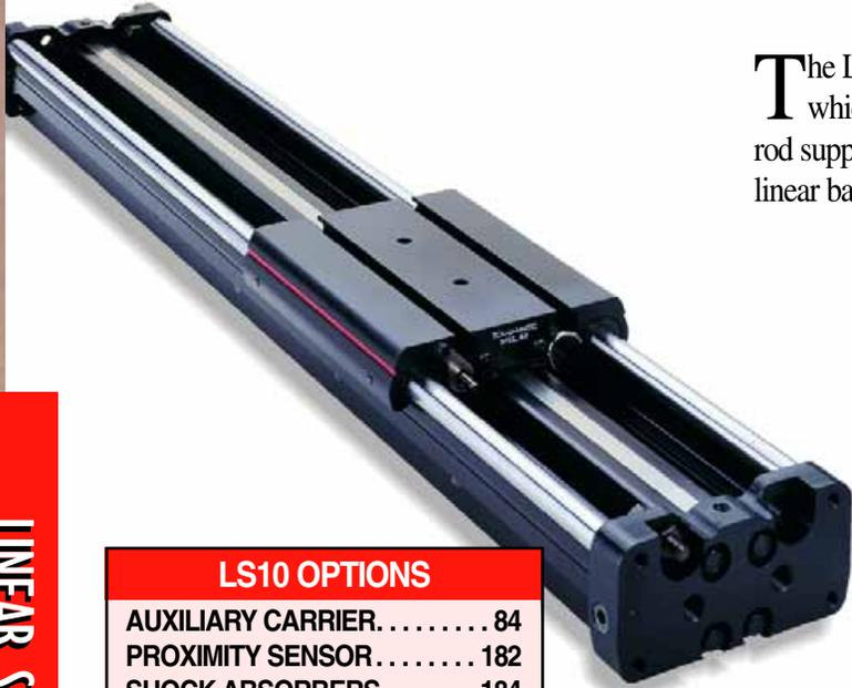
The LS10 features a one-piece extruded anodized aluminum housing which increases torsional stability and provides continuous bearing rod support through the full stroke length. This model features precision linear ball bearings allowing the slide to operate in any attitude.
