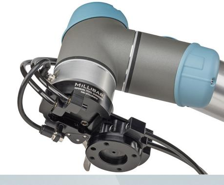
The Utility Series provides dual-channel pneumatic pass-through to control double acting cylinders and grippers. Pass line pressure air for venturi vacuum grippers and part release. Pass 24 VDC signals from sensors and switches on your EOAT back to the robot controller via the 8 Pin M8 threaded male connector that connects to the 8 Pin connector on the UR wrist.
