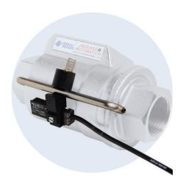
The VA Series valve can be provided with magnetically driven limit switches and an LED indicator. The limit switches are fixed to the outside of the unit. The magnets are situated inside the valve and must be installed during valve assembly, for this reason the switches must be requested at the time of order.
