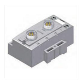
Version Bus coupler Ambient temperature min./max. -10 ... 50 °C Operational voltage electronics 24 V DC -10% / +10% Electronics voltage tolerance Power consumption electronics 0.11 A 24 V DC Operating voltage, actuators Total current for actuators 4 A Protection class IP65 32 Number of solenoid coils max. Number of valve positions max. 32 Undervoltage Diagnosis
