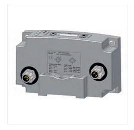
Ambient temperature min./max. -10 ... 50 °C 24 V DC Operational voltage electronics Electronics voltage tolerance -10% / +10% Power consumption electronics 0.1 A Operating voltage, actuators 24 V DC Total current for actuators 4 A IP65 Protection class Number of solenoid coils max. 32 Number of valve positions max. 32
