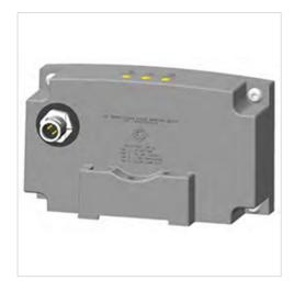
Version Bus coupler Ambient temperature min./max. -10 ... 50 °C Operational voltage electronics 24 V DC -10% / +10% Electronics voltage tolerance Power consumption electronics 0.04 A 24 V DC Operating voltage, actuators Total current for actuators 4 A Protection class IP65 32 Number of solenoid coils max. Number of valve positions max. 32
