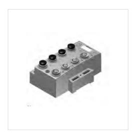
I/O module version Version Ambient temperature min./max. -10 ... 50 °C Operational voltage electronics 24 V DC Electronics voltage tolerance -10% / +10% Max. current per channel 0.15 A 24 V DC Power supply for actuators Total current for actuators 4 A Protection class IP65 Total current of sensors max. 1,2 A Diagnosis Short circuit I/O connection M12x1, 4-pin Weight See table below
