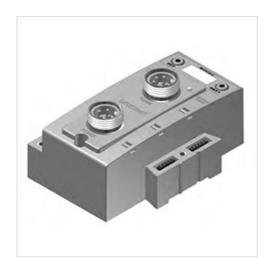
Version Bus coupler Ambient temperature min./max. -10 ... 50 °C Operational voltage electronics 24 V DC -10% / +10% Electronics voltage tolerance Power consumption electronics 0.11 A 24 V DC Operating voltage, actuators Total current for actuators 4 A Protection class IP65 32 Number of solenoid coils max. Number of valve positions max. 32 Diagnosis Undervoltage
