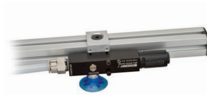
Angled Bracket holds NVP10-60M vacuum generator and cup, with exposed fastening screw for quick and easy adjustments.
