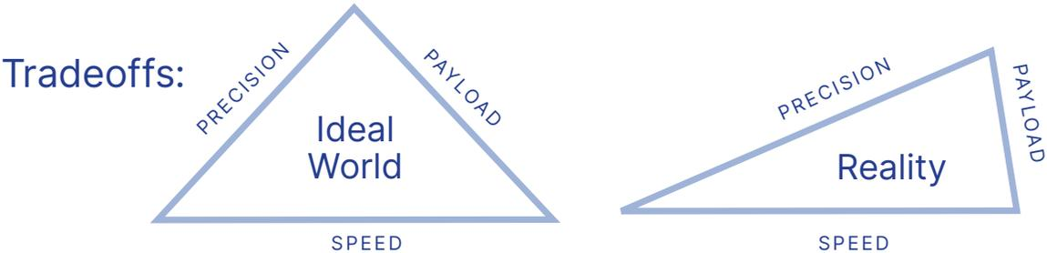
The underlying cause of these performance tradeoffs is vibration of the robot arm. Take, for example, the objective of reducing cycle time — a priority for many manufacturers as they seek to increase throughput and reduce costs. The easiest, and in many cases, most effective way to reduce cycle time is to increase the robot's speed and acceleration.
