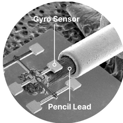
Gyro sensors are used in devices such as automobile navigation systems, and typical sizes are relatively large — about the size of a thumb. But Epson's GYROPLUS Technology uses a gyro sensor small enough to balance on the end of a pencil lead.
