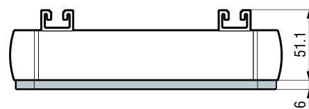
6 mm thick "COVAL-flex" interface
