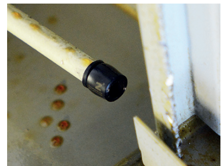
Machine door damping in a machining center
