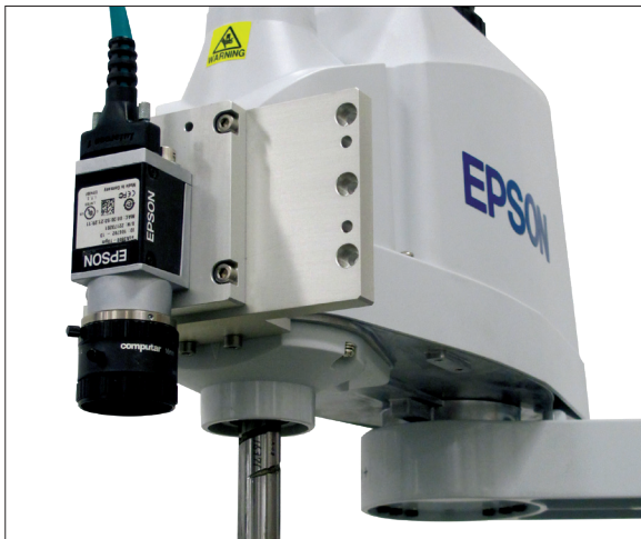
Synthis T-Series shown with mobile mounted camera as part of the Epson Vision Guide option
