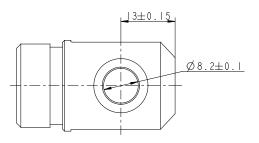
Option "6" Piston 0231016 with bushings, Zinc coated steel
