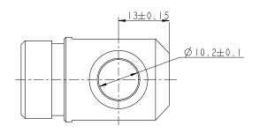
Option "D" and "E" Piston 0301244 with bushings, Stainless steel AISI 304 Piston 031923 with bushings, Stainless steel AISI 303
