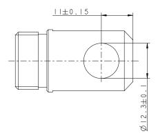
Option "5" and "C" Piston 0231033 with bushings, Zinc coated steel Piston 0231096 with bushings, Stainless steel AISI 304
