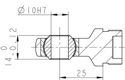
\* With piston rod eye version 'K' the BID is standard plus 11 mm
