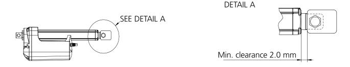
With Zero Point the minimum stroke is 70 mm.
