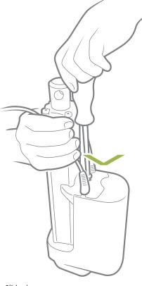
3. Slide the cover onto the actuator.
