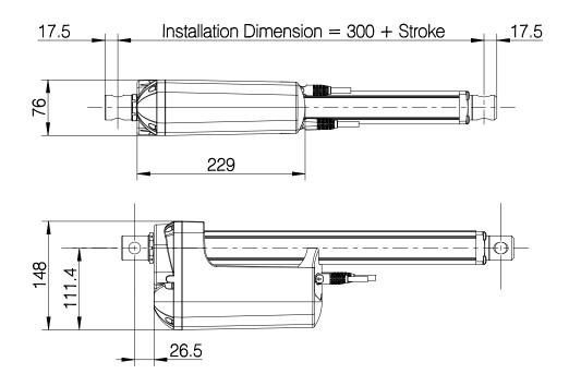
The above dimensions apply for all LA37 piston rod eyes and back fixtures.
