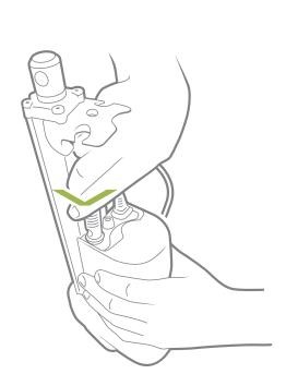
2. Plug in the power cable and/or the signal cable.
