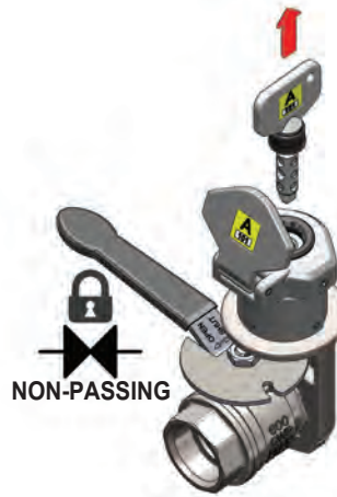
FCL: KEY FREE, VALVE CLOSED
