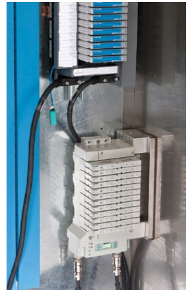
Example: Valve systems connected to intrinsically safe I/O baseplate
