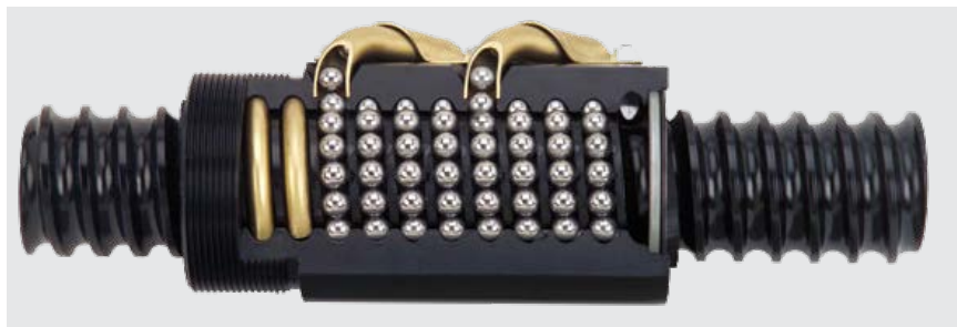
Ball screws are ideal for low-duty-cycle applications with moderate force requirements and moderate to high speeds. A ball screw's ball bearings have fewer points of contact than roller screws, resulting in a lower life expectancy.
