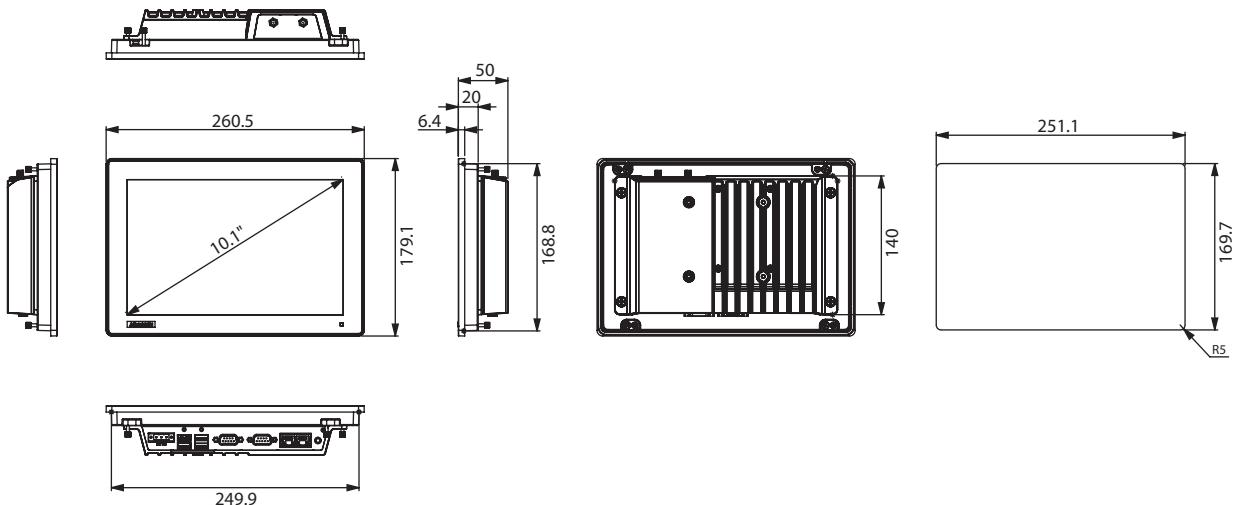
Panel Cutout Dimensions: 251.1 x 169.7mm, corner=R5mm ( $\pm 0.5\text{mm}$ )
