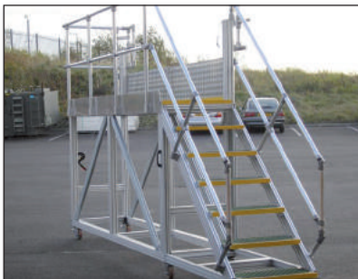
Flask inspection platform
